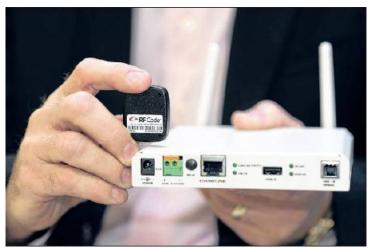
Austin's RF Code makes the hardware and software for wireless sensor networks that monitor humidity and temperature inside big data centers and then send alerts when trouble spots show up. The modules on the left receive signals from a router.
