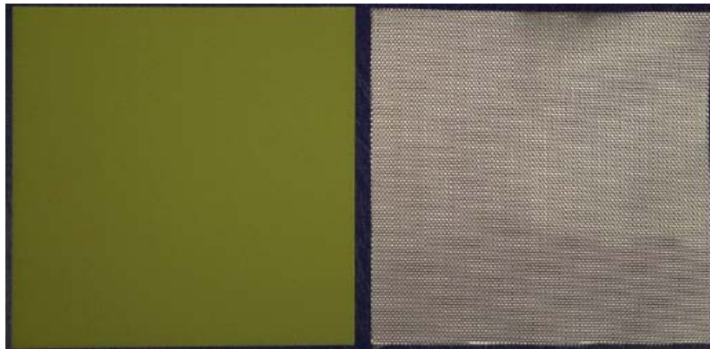
Images of a coupon before (left) and after (right) resin burn off at 538C for one hour.
