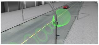
Upon system activation, communication is relayed from the Connected Vehicle Interface unit to the RSU, which transmits data to connected vehicles within range.
