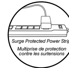
Connect the AC Power Supply to the Connect 4G then to a surge protected AC power strip with at least a 1000 Joule rating. If your Connect 4G is working correctly, the lights will be green.
