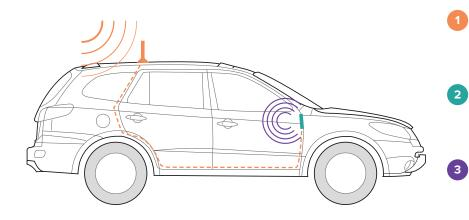
Receives signal: The powerful antenna reaches out to access a voice and 3G data signal, and delivers it to the booster.
