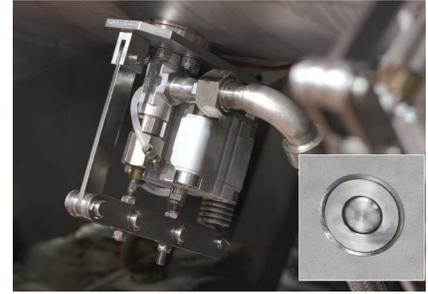
Installed hygienic KRYOJECTOR injector, with view inside the mixer (inset).
