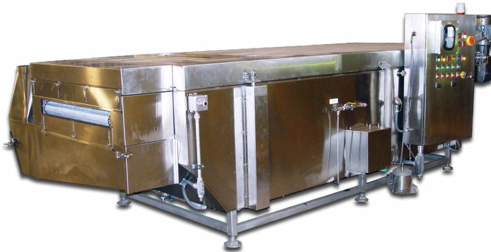
From chicken breasts to pizza toppings, strawberries to shrimp, the Messer nitrogen immersion freezer is the most reliable, accurate, and versatile compact freezer available for processing 1,000-15,000 lb/hr of individually quick frozen (IQF) food. Immersion freezing is the fastest way to freeze while locking important nutrients, moisture, and flavor into the food. The Messer immersion freezer can be adapted to specific processing needs to help increase the quality of frozen product.
