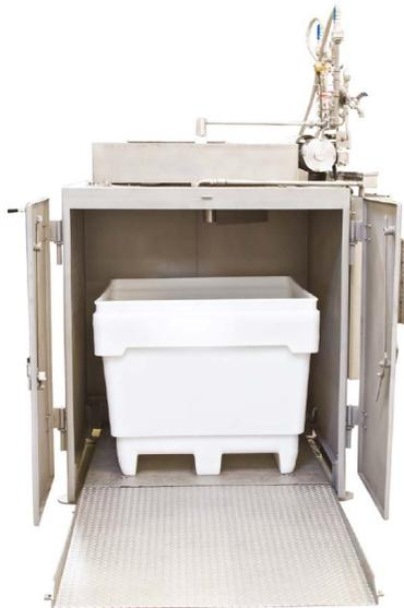
Rapid chilling provided by the Messer combo chiller inhibits bacterial growth that can compromise food quality and safety. The combo chiller supports various types of bins including cardboard and plastic (pictured).
