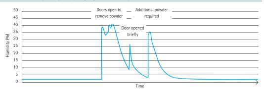
Opening the powder cabinet door and mapping the effect of this on humidity levels. Purging effectively and rapidly reduces humidity even if this stabilization process is interrupted by an operator opening the door again.
