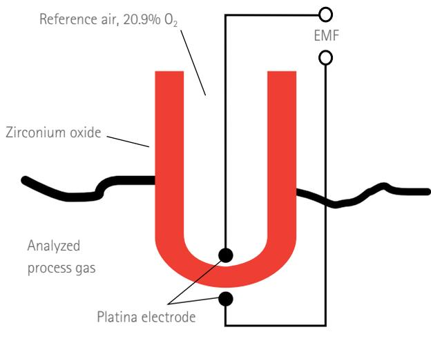
To measure the oxygen content, Nernst's equation (1) is used where  $PO_2(X)$  is the oxygen pressure which is to be measured.  $PO_2(REF)$  is the reference pressure which in this case is 0.209 as the reference gas is represented by the ambient air.  $T$  is the absolute temperature in Kelvin and  $C_1$  and  $C_2$  are constants.
