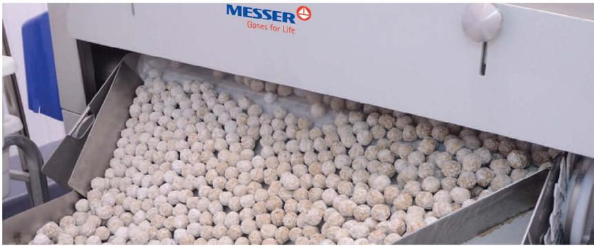
*Pocino Foods quick freezes meatballs, pizza crumble and sliced and diced meat with the new Messer Wave Freezer from which features a patented rolling-wave action to keep products separate as they freeze.*
