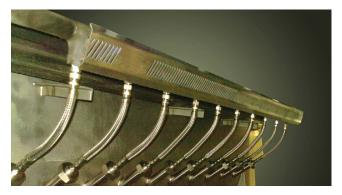
The bottom-injection chilling system on the 10,000 lb/hr meat blender at Interstate Meat uses liquid nitrogen (LIN) and was optimized by Messer. Interstate realized significant "cost to chill" savings with the LIN BI system which cuts chill times by 50%.
