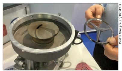
A Varioplast Turbotherm system applied to a Mercedes star emblem mold cavity.
