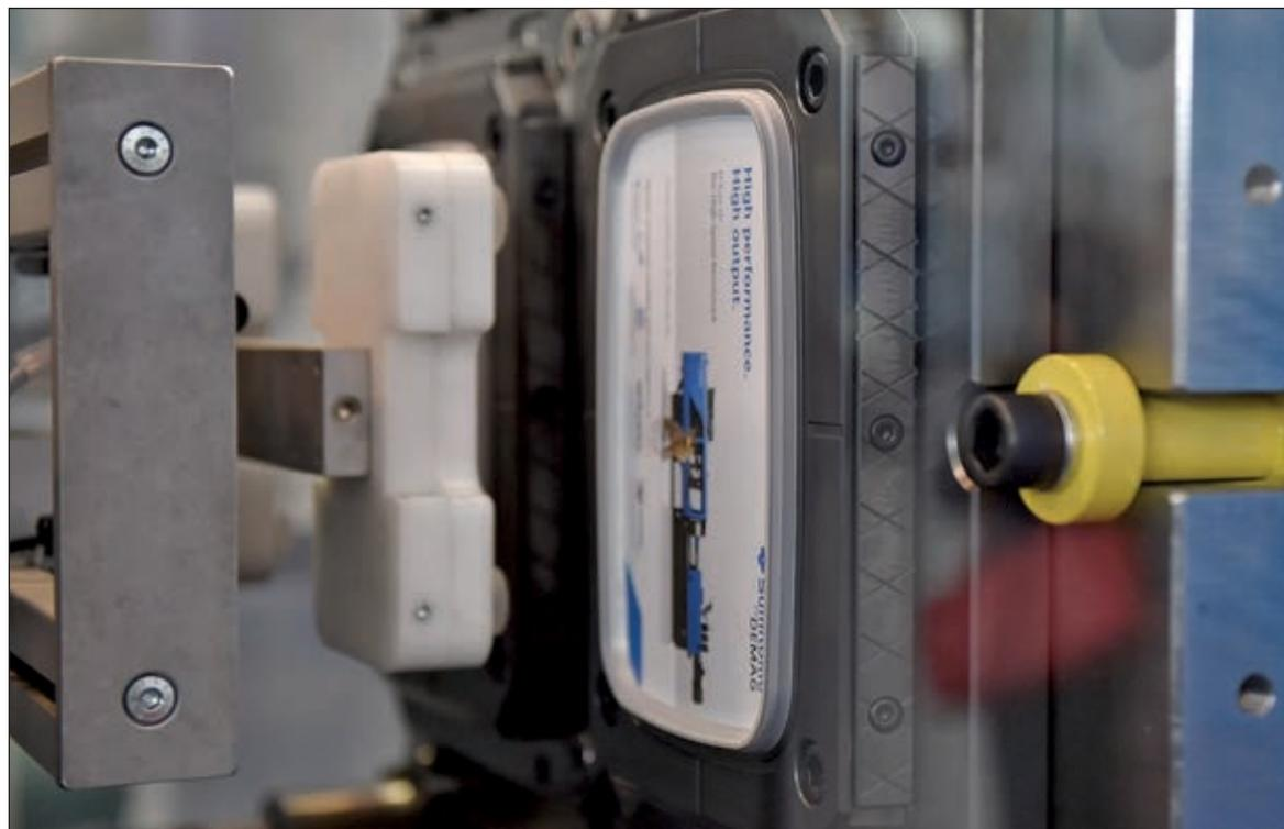
A very thin plastic container cover from Sumitomo Demag Plastics Machinery GmbH.
