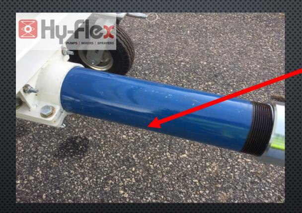
5. With the pipe wrench (minimum 36") unscrew the stator tube from the frame counter clockwise. The stator tube is threaded into the frame and must be removed from the frame BEFORE REMOVING FROM THE ROTOR
