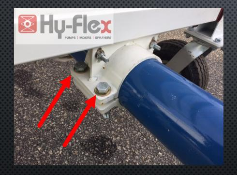
**3.** BREAK LOOSE THE 2 NUTS AND BOLTS USING A <sup>3</sup>/4" SOCKET AND <sup>3</sup>/4" WRENCH. THEY DO NOT NEED TO BE REMOVED.
