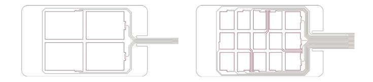
Discrete sensors provide an economical and sometimes more robust alternative to the matrix style sensor. In most medical and industrial applications, a cost effective discrete touch point sensor will better handle harsh user environment, prevent false touches, require less development time and be more cost effective than a matrix style sensor. For these reasons, discrete style sensors are becoming more popular.
