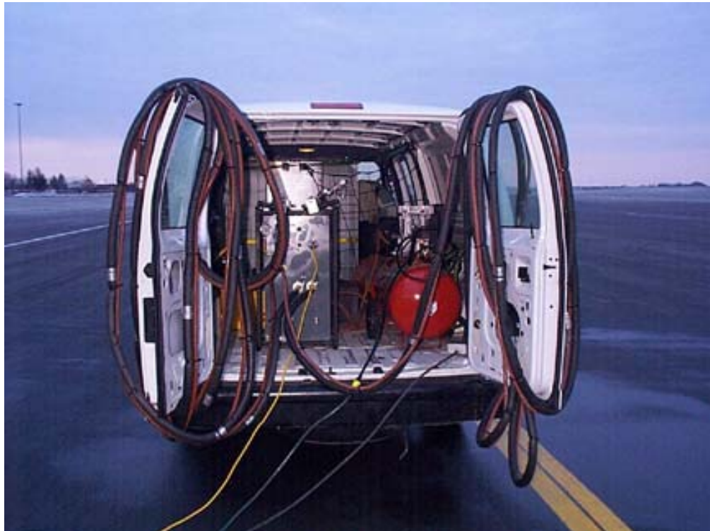
Photo 2.14: Freezing Rain Sprayer with Hoses
