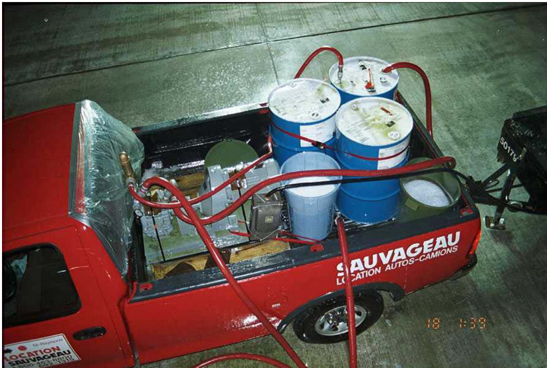
Photo 2.11: Mobile Type IV Fluid Sprayer Unit
