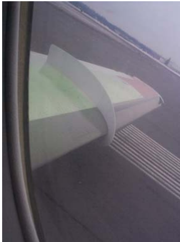
Photo 2.8: Appearance of Type IV Fluid During Taxi
