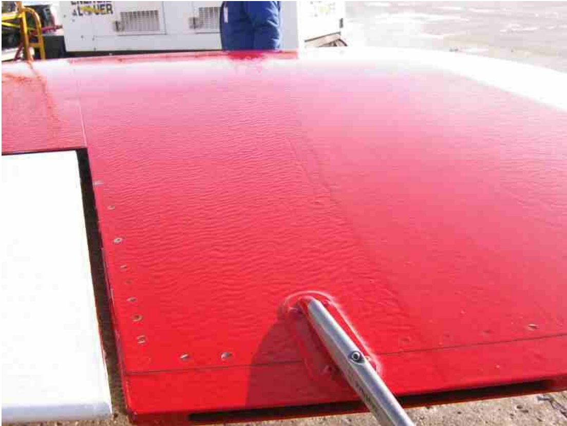
Photo 4.1: Residual Fluid on Trailing Edge
