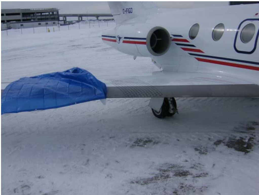
Photo 2.4: Tarp Used to Protect Wing Sections From Fluid Application
