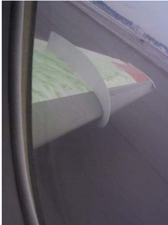
Photo 2.9: Appearance of Type IV Fluid During Takeoff
