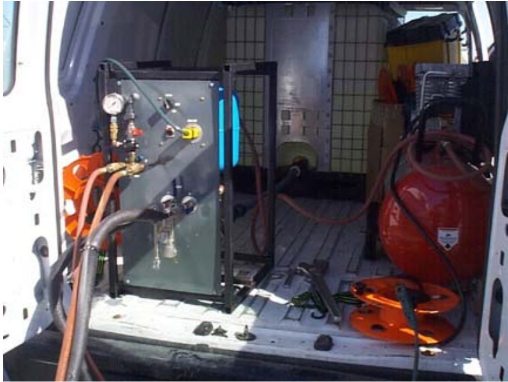
Photo 2.13: Freezing Rain Sprayer
