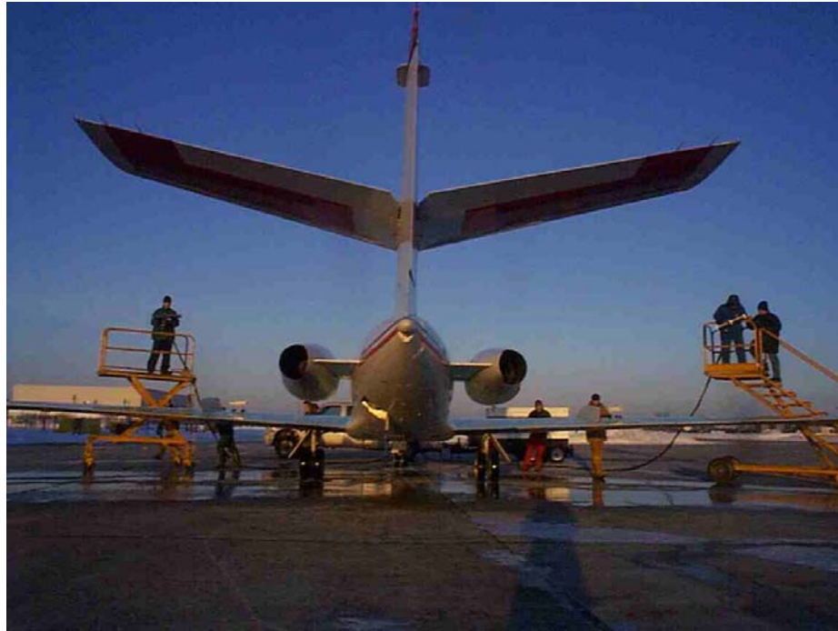
Photo 2.7: Light Freezing Rain Sprayed on Falcon 20
