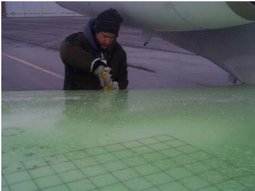
Photo 2.6: Sample Collection for Viscosity Analysis
