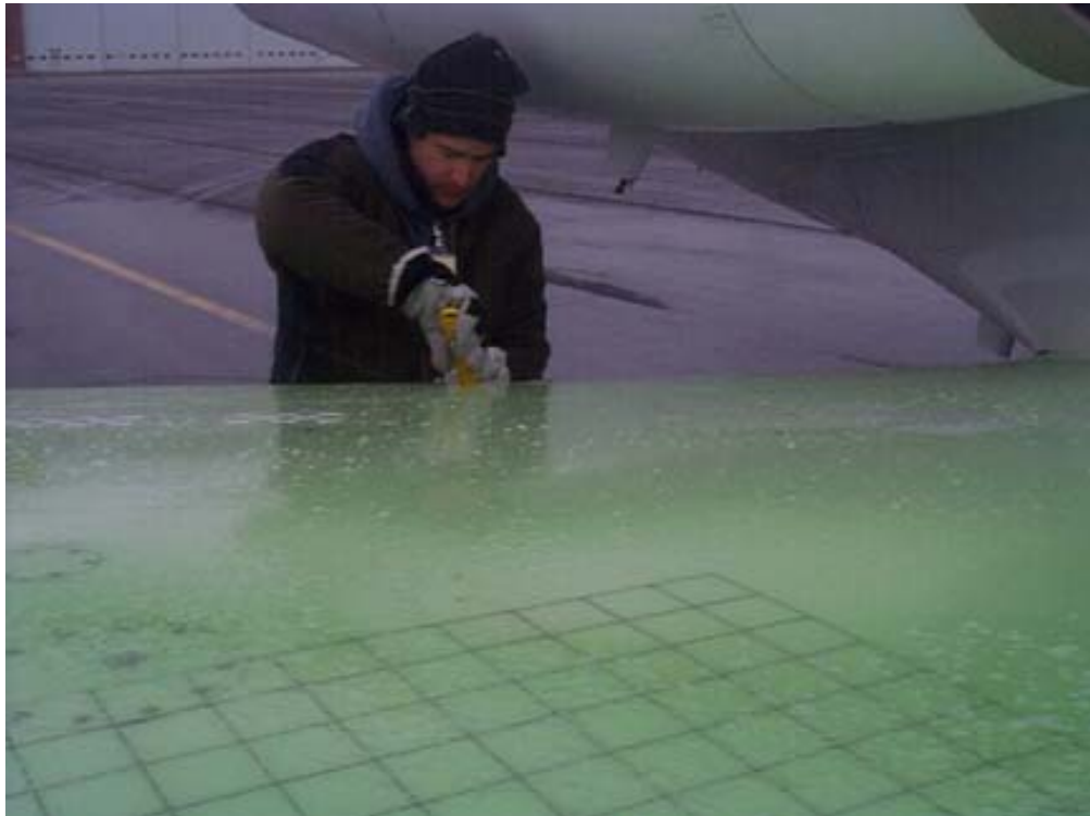
Photo 2.6: Sample Collection for Viscosity Analysis
