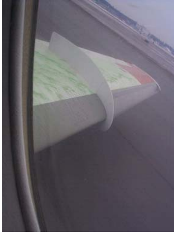
Photo 2.9: Appearance of Type IV Fluid During Takeoff
