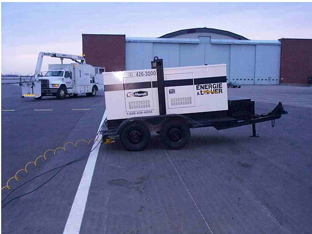
Photo 2.12: Generator Used to Power Mobile Sprayer Unit
