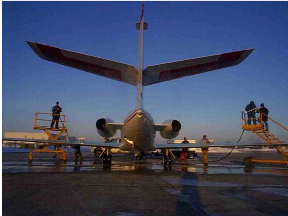
Photo 2.7: Light Freezing Rain Sprayed on Falcon 20
