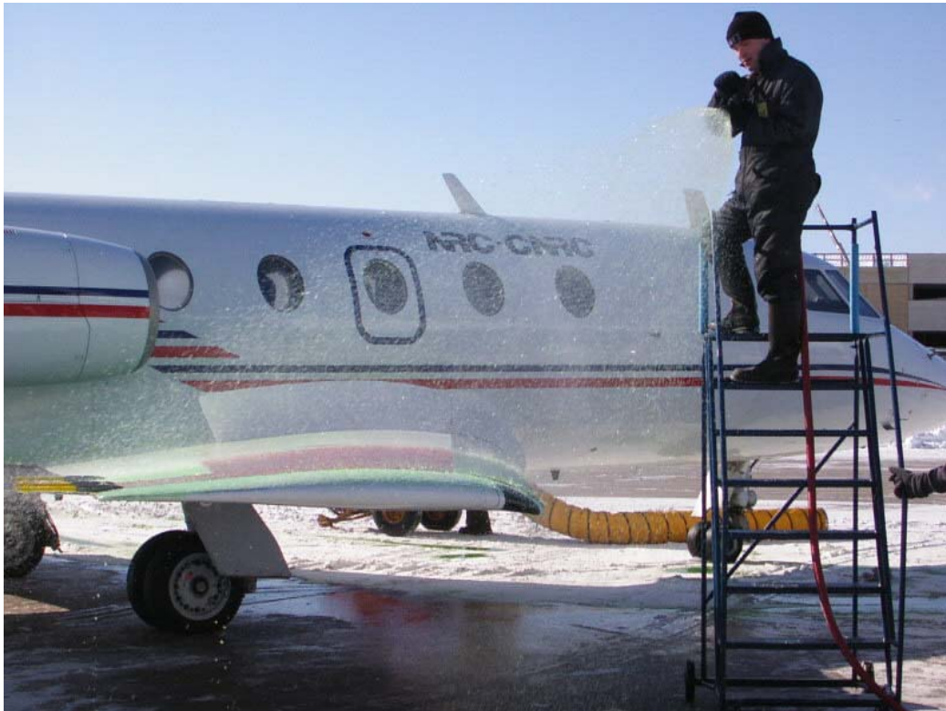
Photo 2.5: APS Personnel Applying Type IV Fluid Using the Mobile Sprayer
