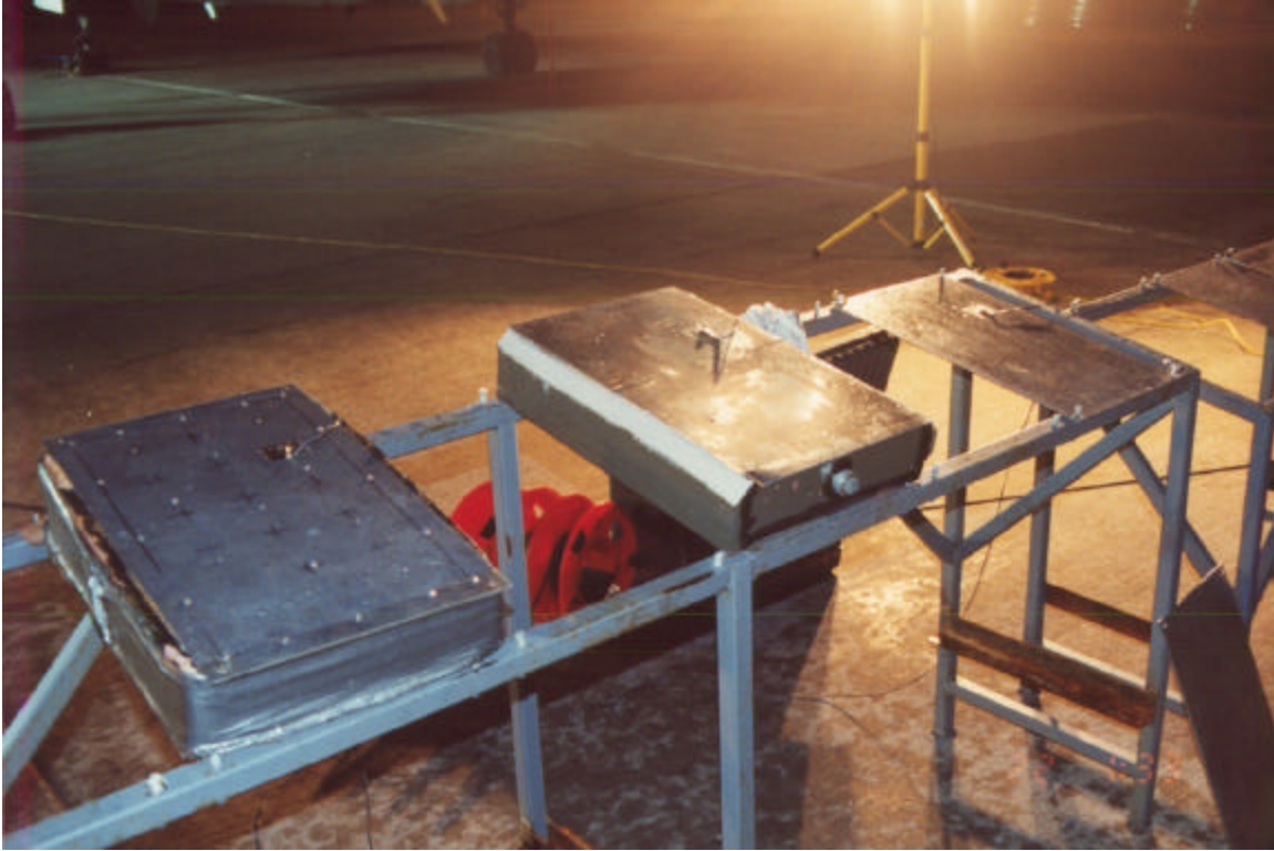
Photo 2.5 7.5 cm Cold-Soak Boxes and Aluminum Test Surface Ready for Testing
