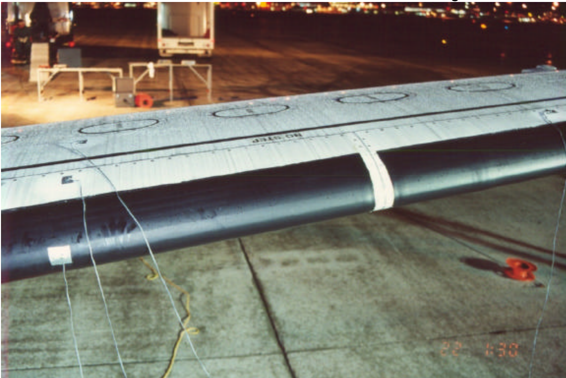
Photo 2.4 Thermistor Probe Installation on Saab 340 Wing
