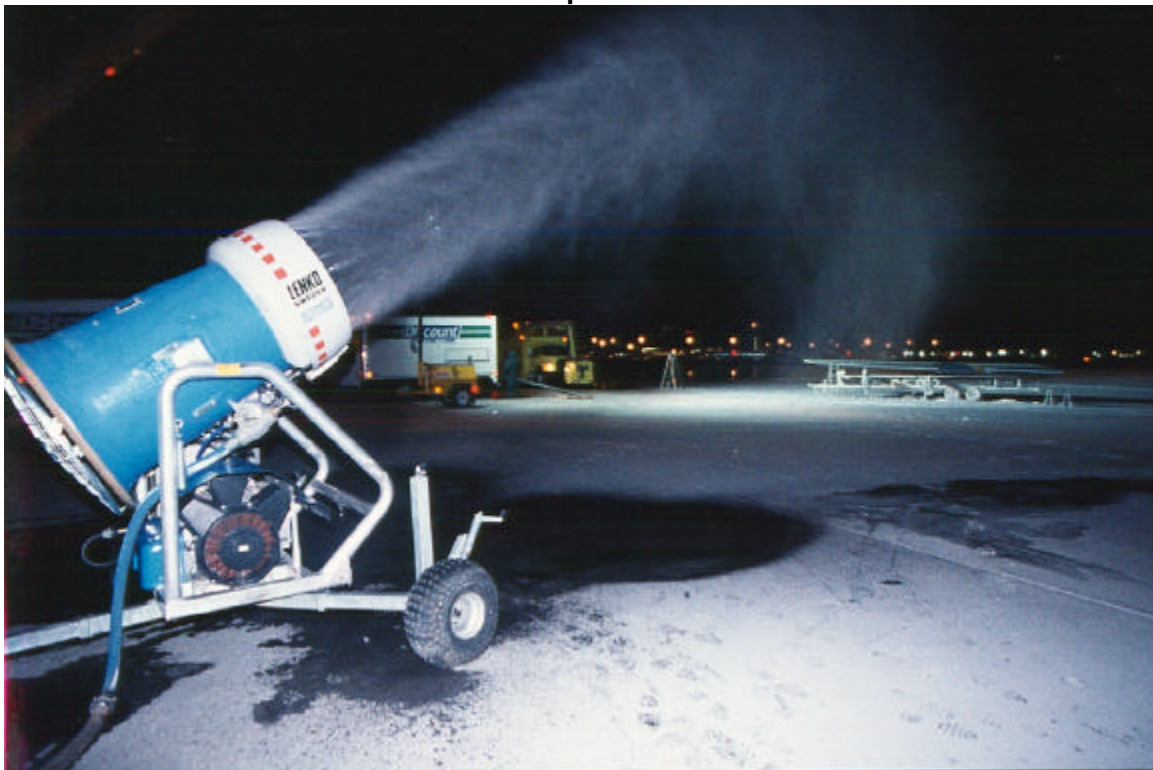
Photo 2.2 Snow Gun Tilted for Improved Snow Distribution
