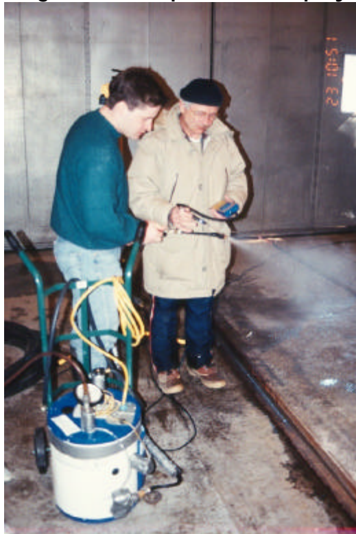
Photo 3.13 Measuring Water Temperature at Spray Nozzle
