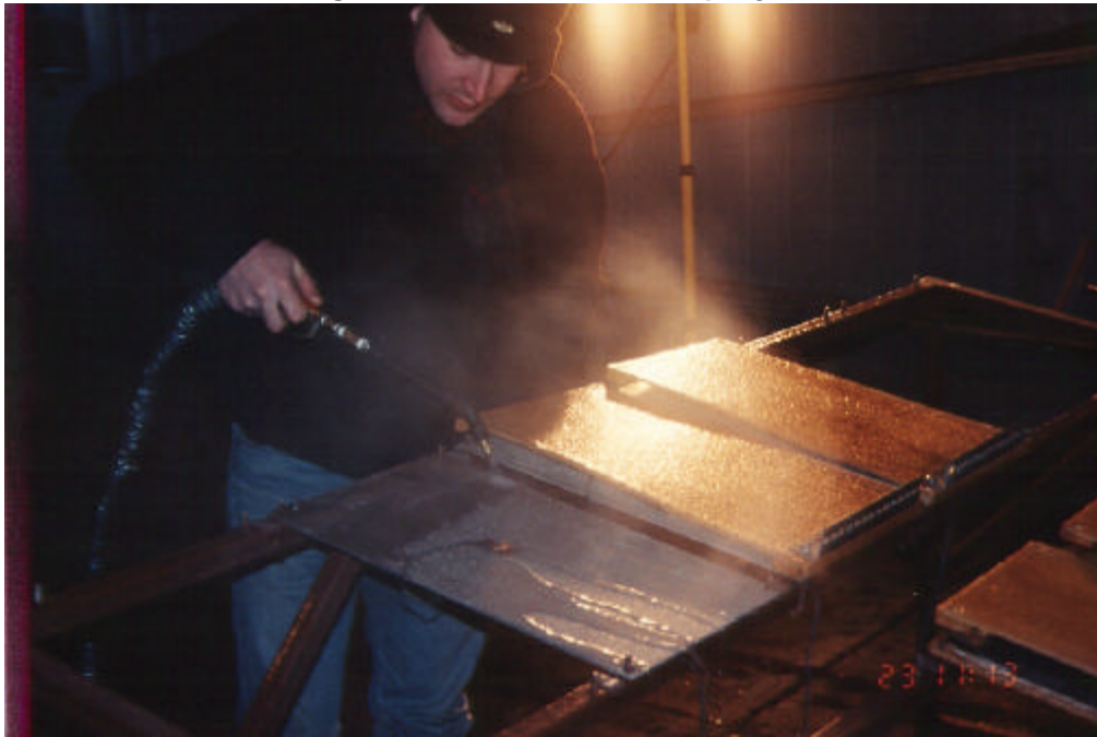
Photo 3.6 Cleaning Ice from Plate with Sprayed Fluid
