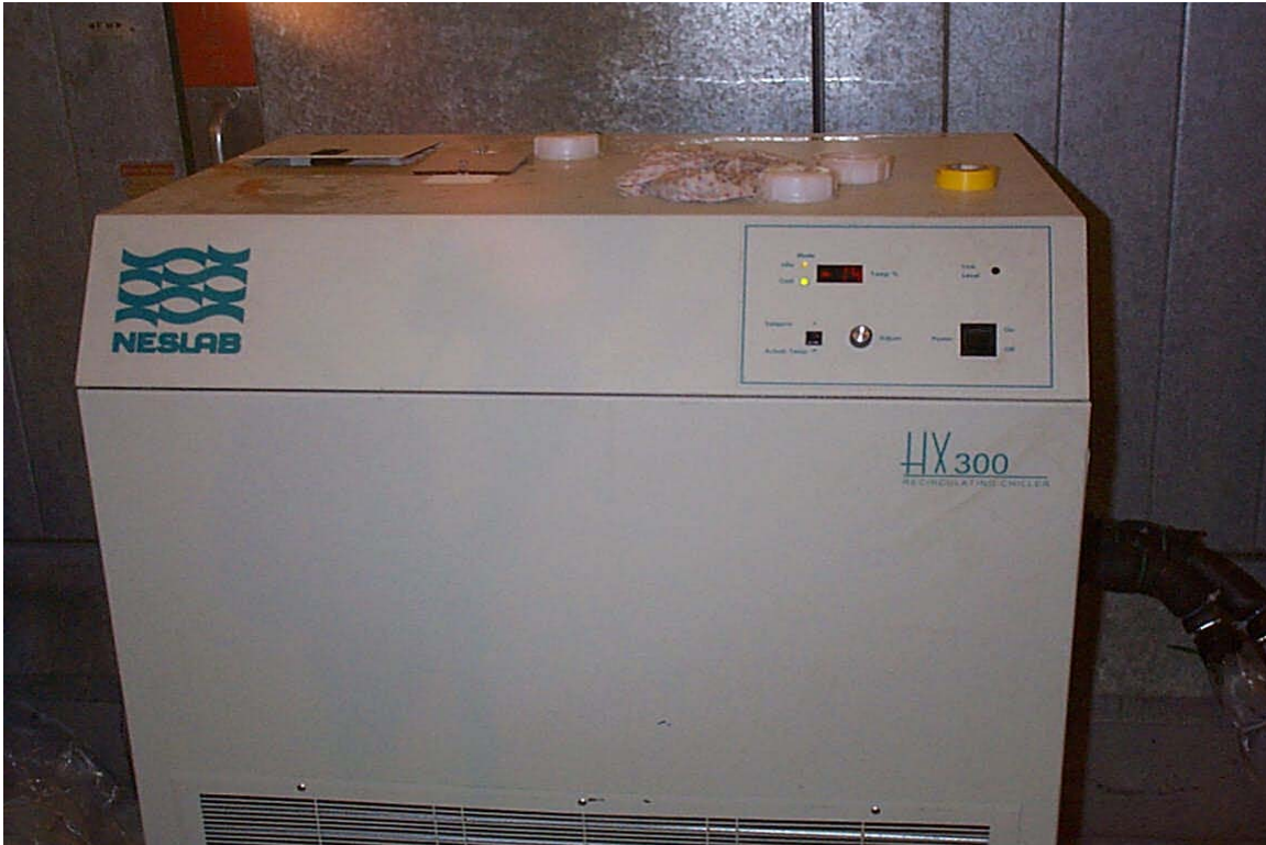
Photo 2.13 New Cooling Unit for Cold-Soak Boxes
