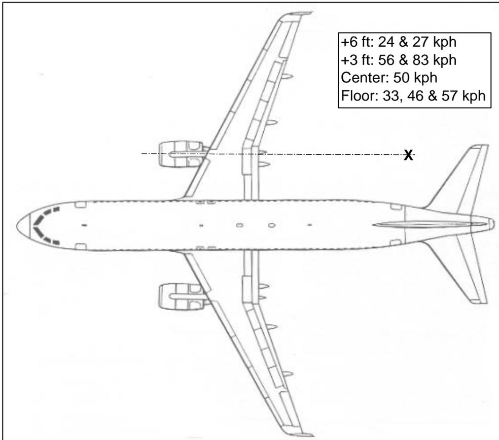
Measurements were taken at an approx. Distance of 8 to 10 ft from LE of the tail.
