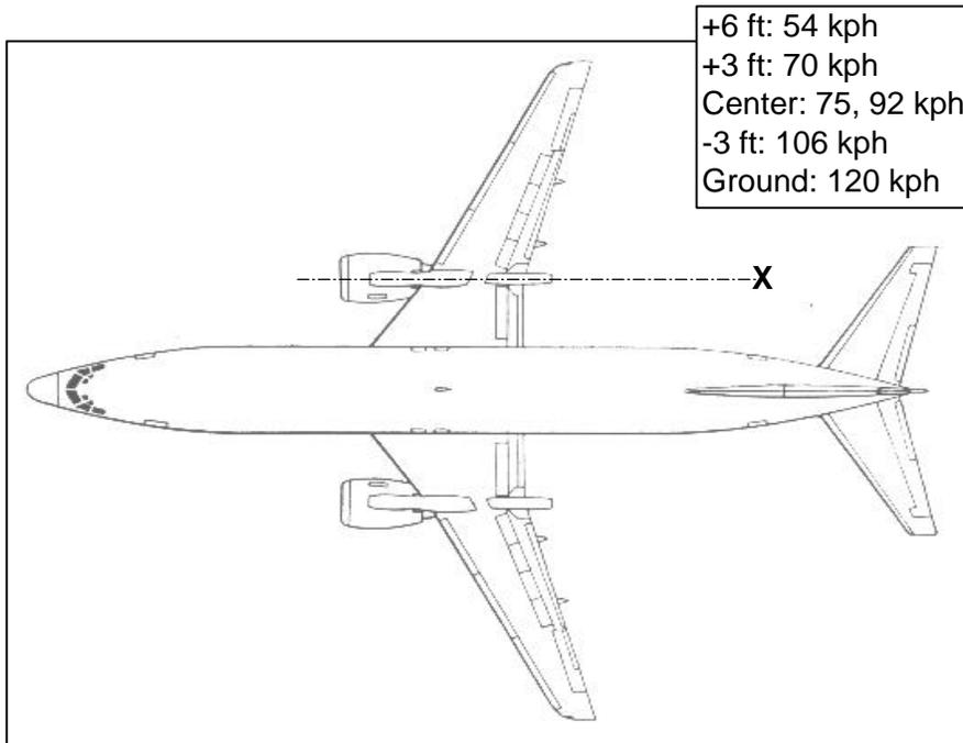
Measurements were taken at an approx. Distance of 8 to 10 ft from LE of the tail.
