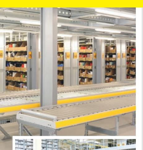
offering storage locations for around 350 000 standard cartons and containers. Around 2.5 km of conveyor technology, roller and belt conveyors and transfer tables connect the different levels and newly set up and linked packing, returns and preparation stations. A load lift was installed in addition to the staircases to allow staff to work on the different levels
