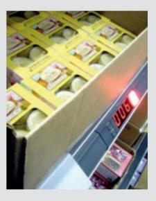
Yankee Candle® provides a huge range of scented candles, produced using the world's most select ingredients. To optimise order picking processes, the company wanted to further develop its existing SSI Schaefer live storage shelving. Integrating a pick-by-light system from the intralogistics specialist has produced the desired result.
