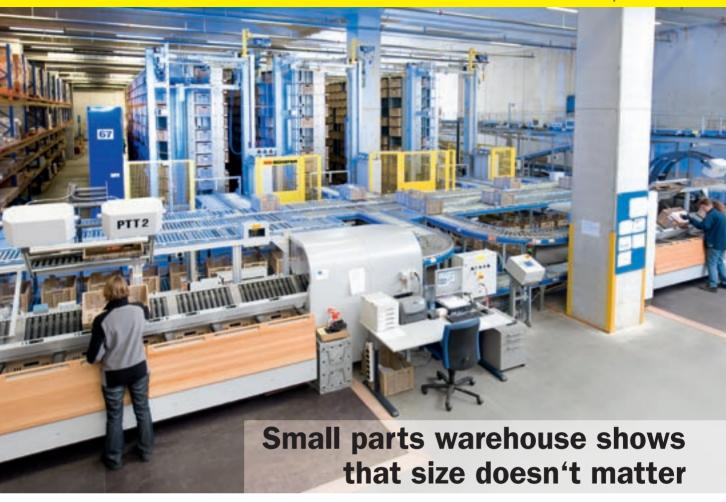
Distribution centre Migros-Verteilbetrieb Neuendorf AG (MVN) was looking to optimise storage and order picking. A "goods to picker" solution now ensures efficient processes. The Schaefer Carousel System (SCS) provides the dynamism needed for order picking with an integrated high-performance order picking workstation.
