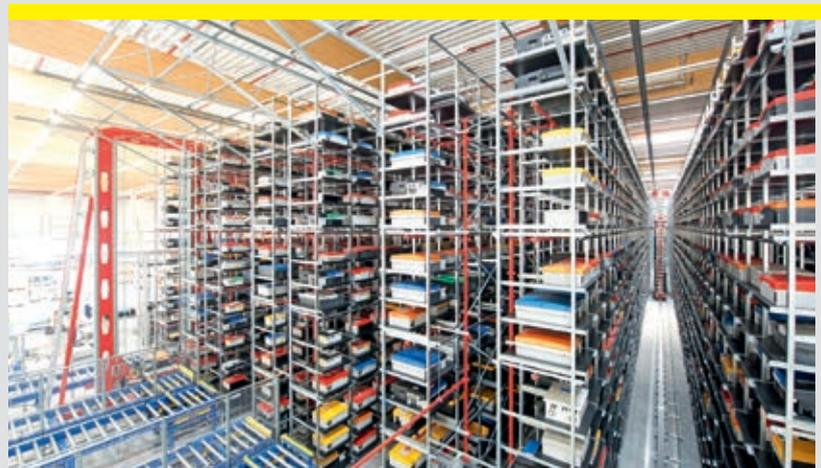
The sophisticated construction of the SMC is geared toward providing the maximum value for the customer. The use of premium steel guarantees high durability and contingency reserves with low costs. Due to the diagonal bracing of the mast, a lower weight, greater elevation and higher throughput are achieved. The design is unique and significant. The traveling unit made with steel-rail and the successful Omega-drive are designed for high availability and low wear.
