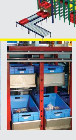
Static as well as dynamic order picking locations can be equipped, for example with Pick by Light.
