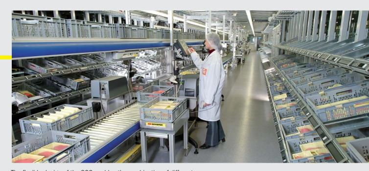
The flexible design of the SQS enables the combination of different solutions, e.g. order picking in flow racks and by "Pick by Light" or the use of static as well as dynamic order picking positions.
