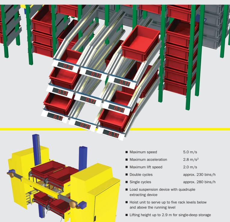
Connection of SQS to other storage areas can optionally be provided by spur tracks (see illus. below) or lifts. The required throughput can be adapted to the relevant needs by the individual number of shuttle vehicles.
