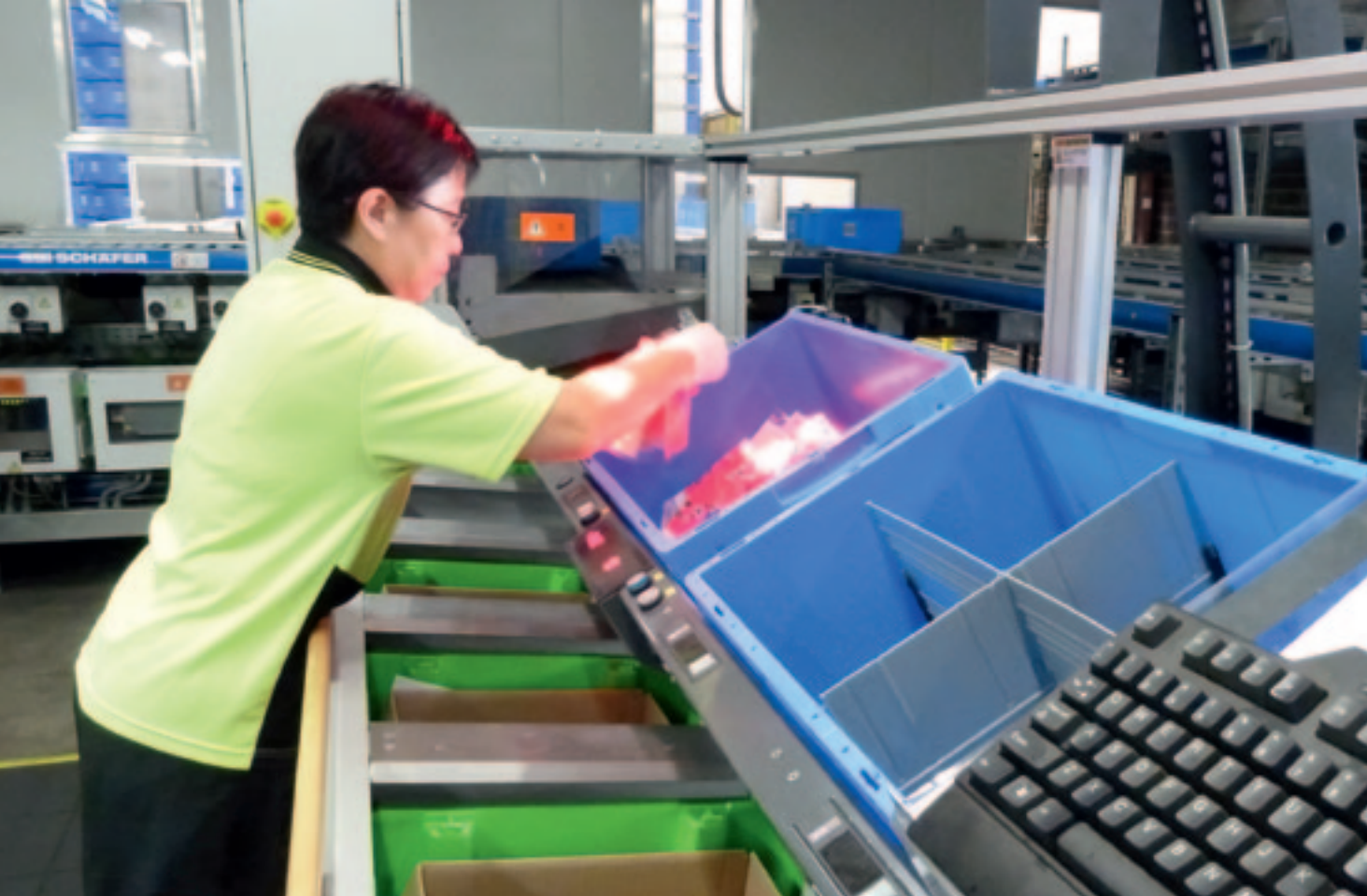
2 pick-to-tote workstations are connected to 6 Schaefer Carousel Systems
