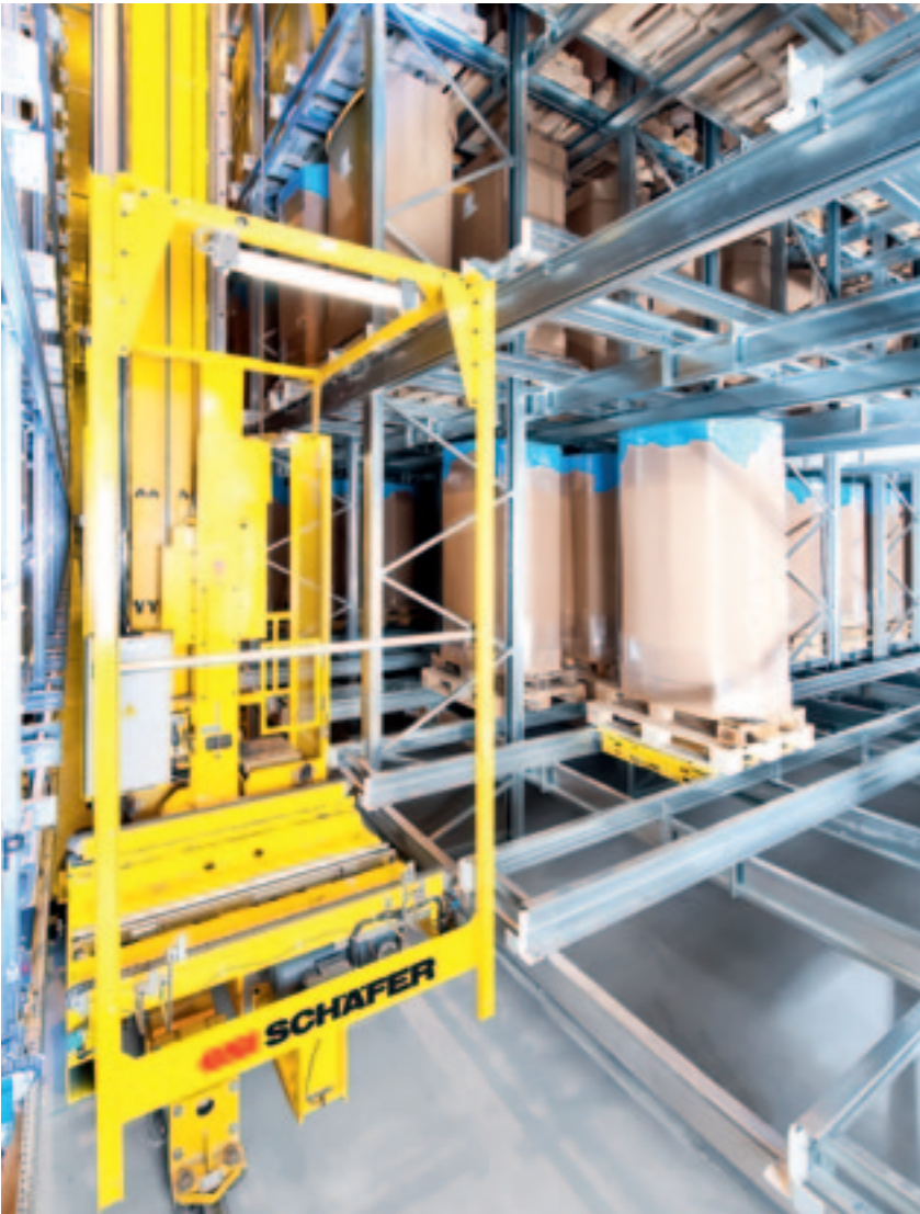
Special combination of the Schaefer Compact Crane storage and retrieval system and the Schaefer Orbiter System as a shuttle solution
