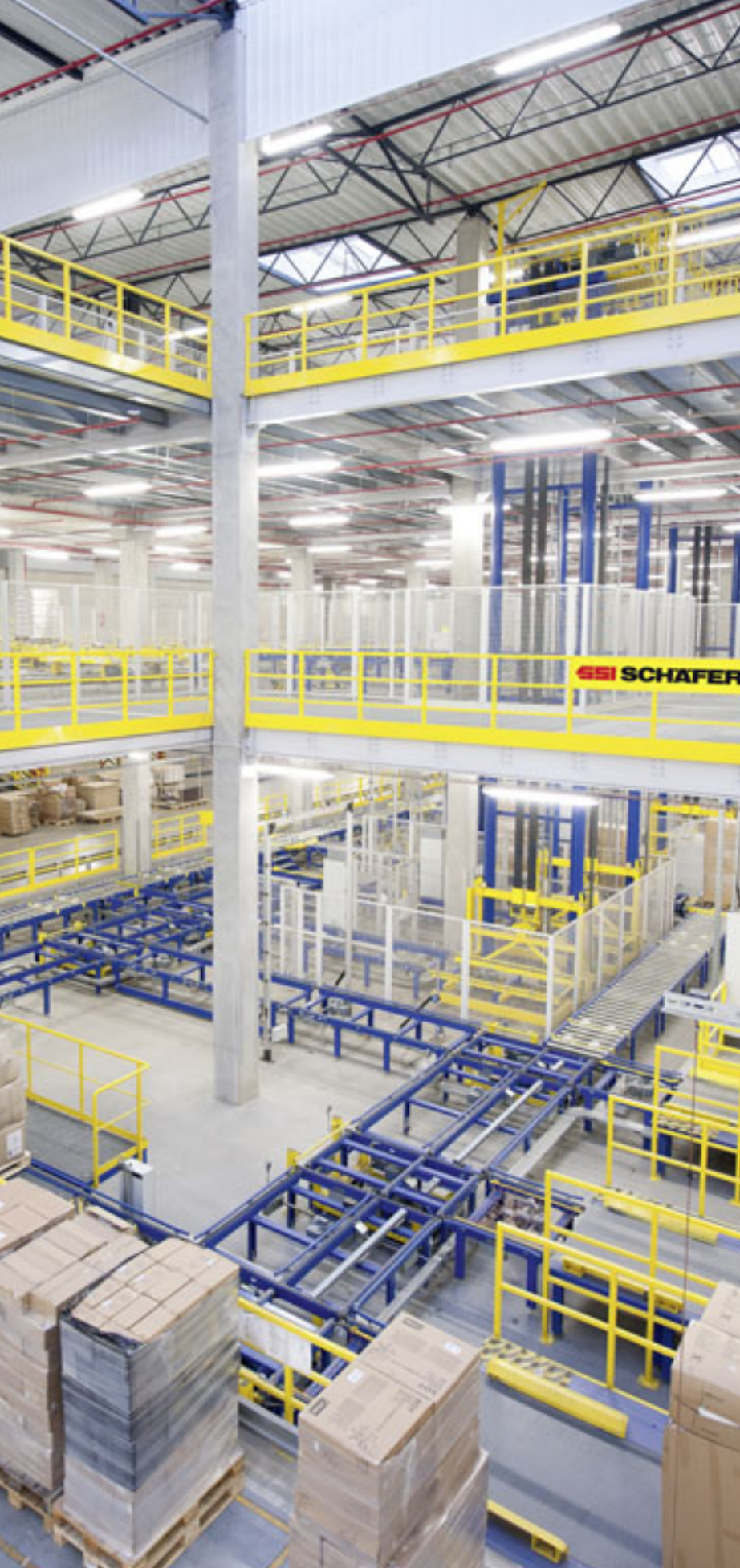
Vertical transfer lifts transport the pallets onto the upper levels for transfer to the electrical pallet conveyor
