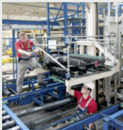
All components of the storage and retrieval system were replaced, except for the mast and undercarriage cross beam.
