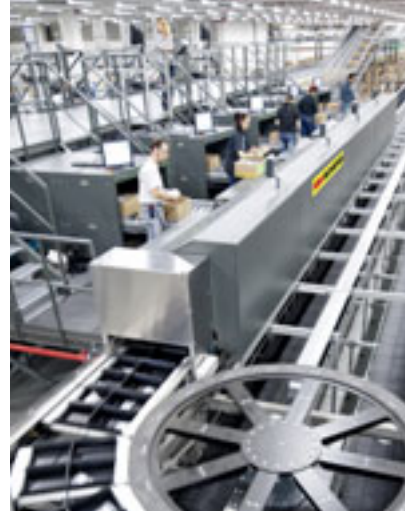
Pick-to-bucket system: Every picking station has a collection system with 16 funnels assigned to it.
