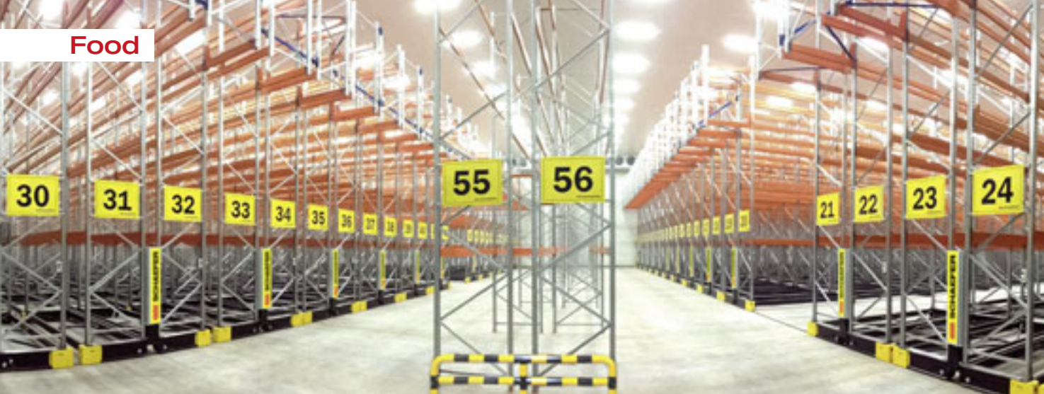
The mobile racking system provides space for 14,500 pallets or for 13,000 tonnes of goods
