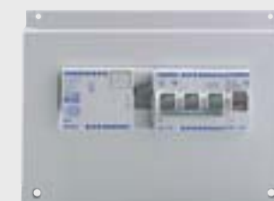
FI-safety switch (4-pole 40A/0.03A), fuse (3-pole 35A), fuse (1-pole 16A)
