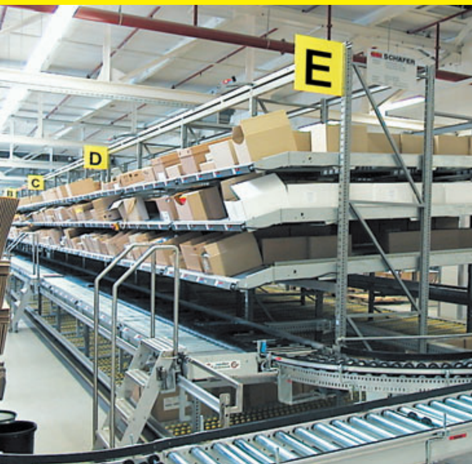
Illustration top: Live storage shelving with integrated material handling and pick-by-light in the publishing industry Illustration bottom: Live storage shelving with integrated material handling and pick-by-light in the pharmaceutical industry
