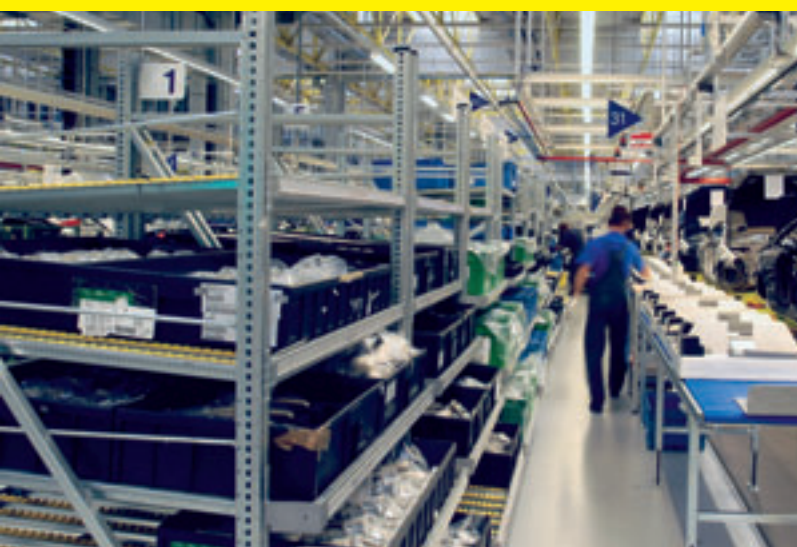
R 7000 on-line shelving with glide rails
