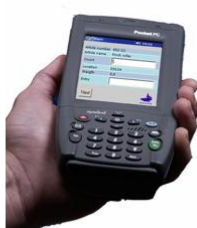
Wireless hand terminal with built-in barcode scanner and SHARK software
