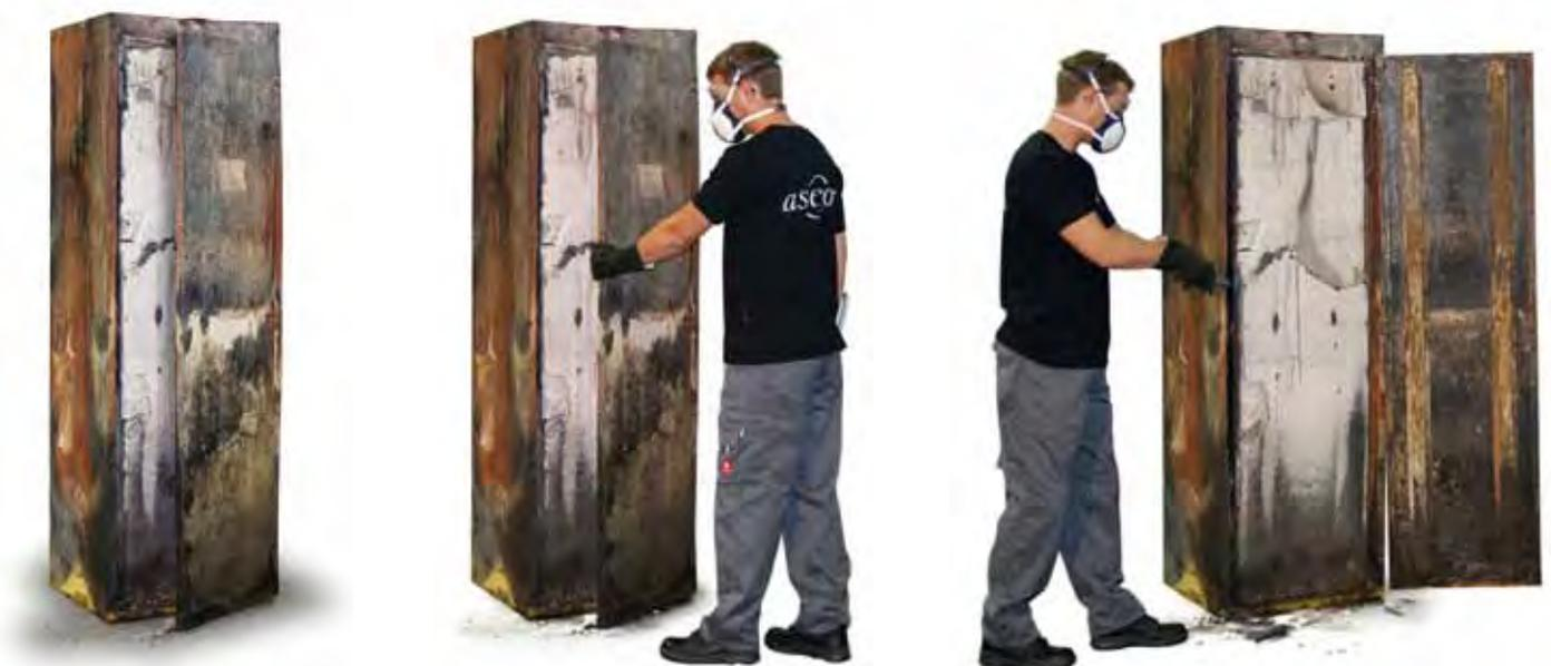
After opening the cabinet, it was possible to salvage all of the hazardous materials inside. Both the plastic containers and the flammable liquids contained in them had been shielded against the heat by the safety cabinet.
