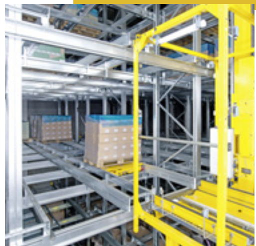
Two tracks for receiving goods transport the pallets to the storage and retrieval system.
