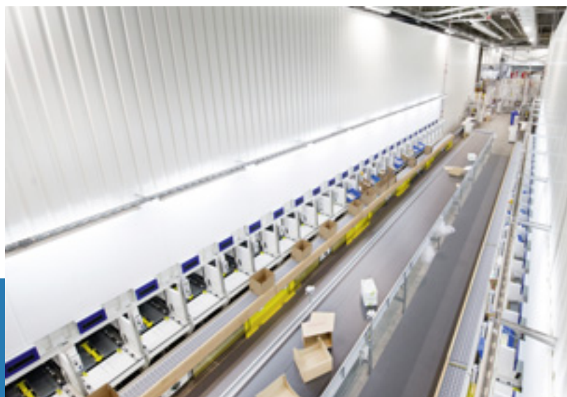
To assemble orders comprising packages of small parts, the trays are moved out to five workstations, each consisting of five picking stations. One picking station is located in front of each of the automated small parts stores.
