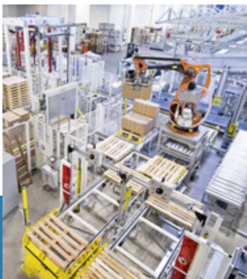
After being automatically strapped and labelled, the shipping boxes are fed to the palletising robots. From there, the newly assembled pallets are transferred to the shipping area.
