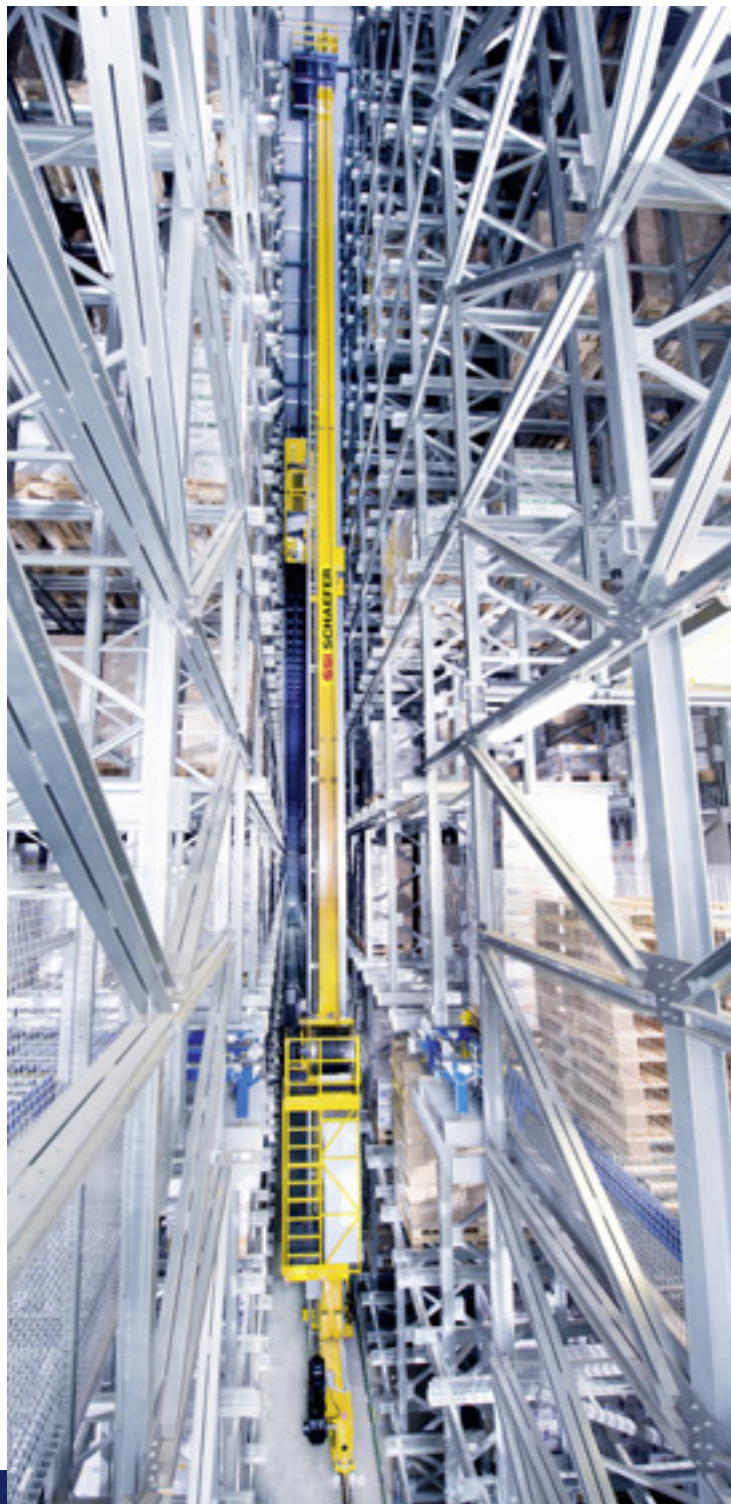
The storage and retrieval machines place up to 52 pallets in the channels each hour and remove up to 126.
