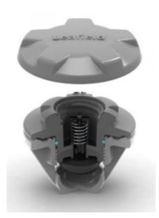
The D7 Valve has improved inflation/deflation speed compared to the C7. It has an improved clamping method, with an '0' ring seal added to the valve core, to reduce the risk of lateral leaks in the fabric.
