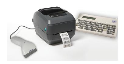
This stand-alone system includes a scanner, keyboard with display, and barcode printer. The scanner reads barcodes directly, and the keyboard allows you to add or modify label information before printing. It is compatible with labels used in demanding conditions, such as Computype Cryo Hold™. Small, affordable and easy to use, the Barcode Duplicator helps you track samples accurately and consistently while reducing time and effort.
