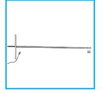
T-handle with 3/8" penetration to check moisture in stacks in or out of kiln. Stickers must be at least 5/8". Also available as the 42-EB/4.5 in 4 1/2' length.
