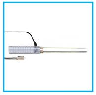
Two insulated 9 1/2" pins with 8 1/4" penetration. Eliminates the effect of surface moisture. Used for bales.
