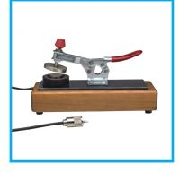
Clamp type for testing thin sheet stock, veneer, and fiberboard between two smooth disks.
