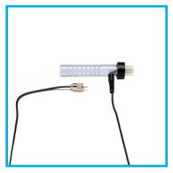
Eight insulated 1 1/2" pins with 1" penetration. Used for yarn.
