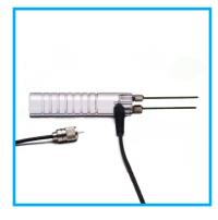
Two pins with maximum 3 1/4" penetration. The pins are insulated except at the tips. Used for roofs, insulation, or EIFS. Also available as the 21-E/001 with 6" penetration or as the 21-ET with a tapped handle for hard to reach areas.
