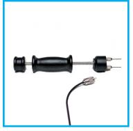
Two pins with 1 1/8" penetration. The pins are insulated except at the tips, which provides much more accurate readings of moisture content.Used to measure moisture content at various depths in plywood, concrete, dry kilns, and hardwood.
