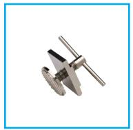
Standard upper electrode assembly for the G-7 moisture meter. The 1900 has a serated face and is used with the 313CUP-0005 cup.
