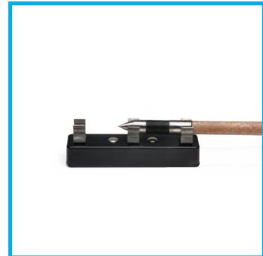
Moisture content standard used to verify moisture meter calibration. Has electrical resistance values of 16% and 22% to test against.
