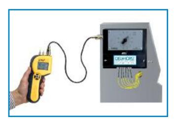
Ideal for conventional dehumidification kilns and small drying operations, KIL-MO-TROL lets you monitor the moisture content of lumber during the drying process. With testing stations at each lumber package and a rotary switch box in your control room, you can quickly obtain an overall view of your progress. Proven for both hardwood and softwood drying, the KIL-MO-TROL can also be used in a pre-dryer or air drying operation.
