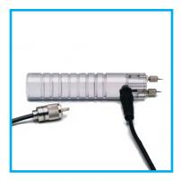
Uses the same contact pins that are mounted on each meter, providing 5/16" penetration. Used on wood up to an inch thick.
