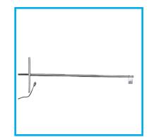
T-handle electrode with 3/8" penetration to check moisture in stacks of lumber in or out of the kiln. Stickers must be at least 5/8". Also available in 4 1/2' length as 42-E/B/4.5.
