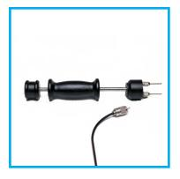
The #496 2" insulated pins on this slide hammer electrode allow you to determine accurate moisture readings at various levels of penetration. Useful for determining moisture gradients in lumber.
