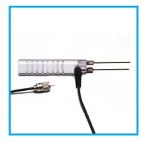
Features #608 4" insulated pins for use on insulation and fooring. Also available for the 21-E are the #608/001 7" extra long insulated pins, ideal for EIFS.
