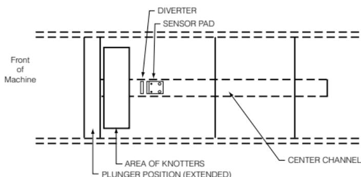
If placing the #1986 in the center channel you may need to cut an opening from the outside to be able to tighten down the nuts and secure the wire or use longer bolts and spacers.
