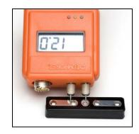
Note: When checking digital wood meter models with the MCS-1, the meter should be set to default: 4-pin, 70°F, Douglas Fir to obtain the nominal 12% and 22% readings. If set to 2-pin, 70°F, Douglas Fir, the readings will be 12.7%, and 23.6%.
