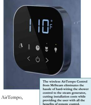
"In a typical installation, you must run wire from the generator behind the wall through conduit to the control, avoiding other wires and high-current devices," explains MrSteam president Michael Pinkus. "With wireless, you <u>avoid</u> all that cutting and routing, as well as the most nerve-wracking process of all: cutting a hole in the shower's marble, tile or granite walls to mount the control and route the cable."
