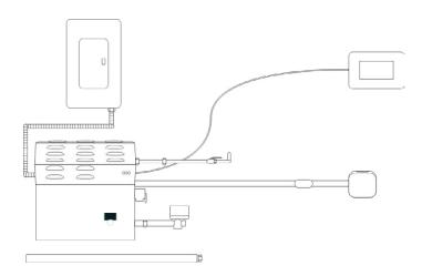
The plumbing connections include a water line to the generator, a steam line from the generator to the steam room, and a drain line.
