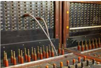
Crosspoint switches originated in telecommunications around 1915 as a way to create a circuit between two phone lines. Originally these were electromechanical devices that used a metal bar to create an interconnect and therefore were known as crossbar switches. Eventually these were replaced by semiconductor technology but the concept remained the same of having a matrix formed from the set of inputs and outputs. (hence also the common name of matrix switches).
