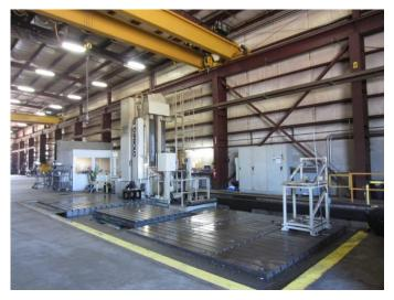
jobs safely and fills a market need for large equipment fabrication. AT&F Wisconsin also houses an enormous floor bar, capable of holding and machining a part up to 51 feet long, 16 feet wide, and 20 feet tall.
