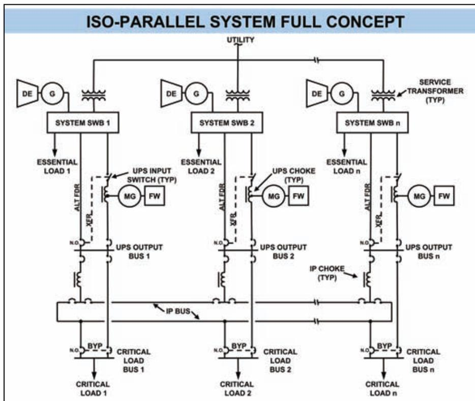
Typically, these configurations have taken one of four basic forms: double-redundant (or system-plus-system) with independent “A” and “B” systems; multi-module parallel-redundant (multiple modules paralleled on a common power bus); isolated-redundant (dedicated modules or systems to act as the redundant unit to all others), and shared-redundant (or distributed redundant) wherein loads are transferred among multiple systems.
