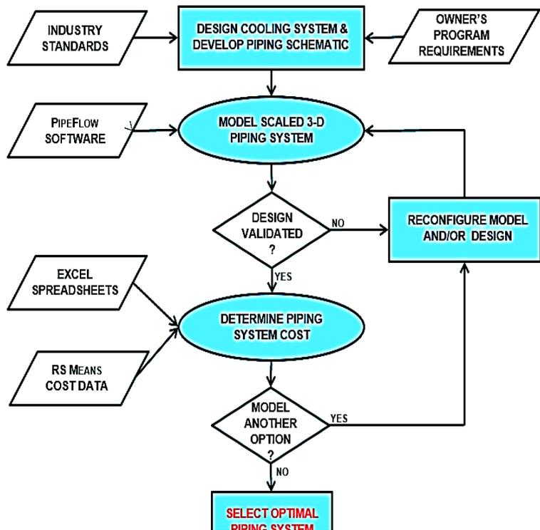
Figure 1: Piping System Design Overview
