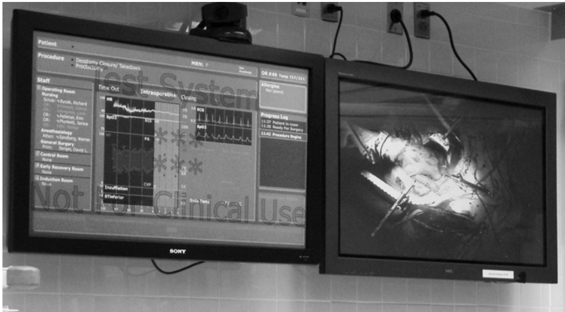
Figure 3 The integrated display resides directly adjacent to the surgical display. The close proximity of two large displays mandated that the design avoid detracting from the pre-existing surgical display, which is often in use during cases. The system is designed to provide adequate size of text and graphical resolution to be visible and legible to anyone in the room, requiring the use of a large 42” LCD display.
