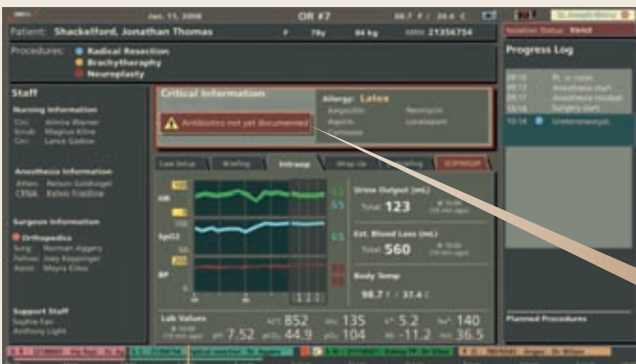
Fig. 4: The OR-Dashboard display, as it appears during the "intraop" phase when antibiotic administration was not documented
