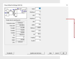
SmartCtrl 4.2 allows the user to define the switches output capacitance (Coss) in order to study the conditions of the zero voltage switching (ZVS).
